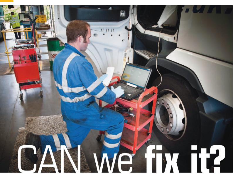
Technicians today are faced with very sophisticated vehicle electronics. John Challen and Richard McLaughlin explain the networks that connect multiple ECUs to manage everything from engine performance to braking and stability – and the role of diagnostics transfer, without electronics or energy consumption
